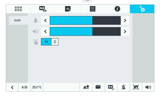
If the user should decide to silence the ring tone of the video door phone, for example while sleeping, it is sufficient to touch the soft touch 2/2 button below. To reactivate the ring tone, touch the 2/2 button again. Otherwise, it is possible to silence the ring tone only for a set period of time. Once the time has expired, the ring
